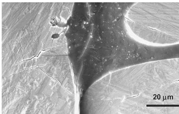
Fig. 6 HZ refractory damage by microcracking observed by SEM after a 1,300 °C heat treatment [6]. Cracks are observed at the interface and within zirconia and glassy phase
